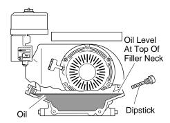
Figure 6 - Checking Oil Level (Model PGH7500IE Shown)
